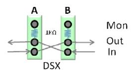
The BTS Master or Cell Master should be set to Terminate Mode when plugged into the DSX-1 Out and In ports. Terminate mode is also used with the RJ-48 jacks commonly used between E1 circuit elements. In either case, a loopback is required somewhere else on the E1 circuit to return the transmitted signal to the test equipment receiver.
