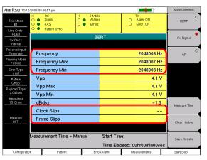
Vpp: Voltage Peak-to-Peak, is a measure of the E1 signal amplitude. This is also measured as dBdsx where 6 Vpp equals 0 dBdsx.
