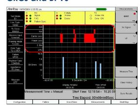
CRC, or the Cyclic Redundancy Check numbers, are included in the PCM30 CRC or PCM31 CRC format. If the received CRC and the CRC calculated from the received data do not agree, the received data must be in error.
